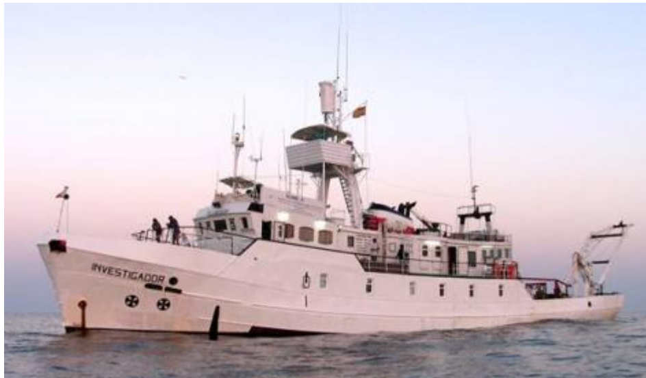
Fig. 1 - A 43m long vessel equipped with a temporary observation platform at about 9m above sea level.
