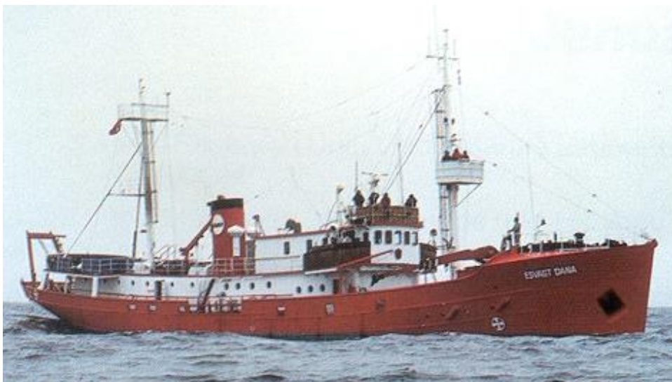
Fig. 2 - A 60 m long vessel equipped with a temporary observation platform at over 10 m on the sea level.
