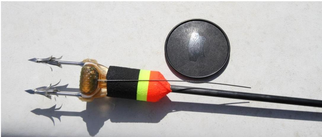
Fig. 1 – Low Impact Minimally Percutaneous External Electronic Tags (LIMPET) tag with anchor system and deployment arrow.
