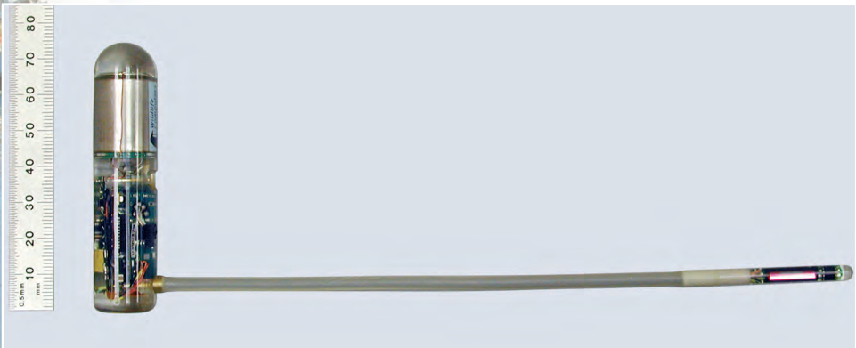
Figure 4. Example of an implanted archival tag (© Wildlife Computers).
