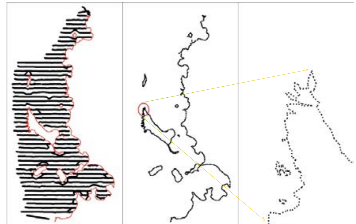
Figure 26 Obtaining zero depth point objects from coastline layer: bathymetry and coastline layers overlaid (left), point objects created for the whole digitized coastline (middle), point objects zoomed (right)
